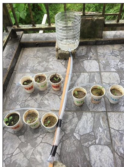
Figure 2. Shows the Irrigation System that was Built to Water the Plant
